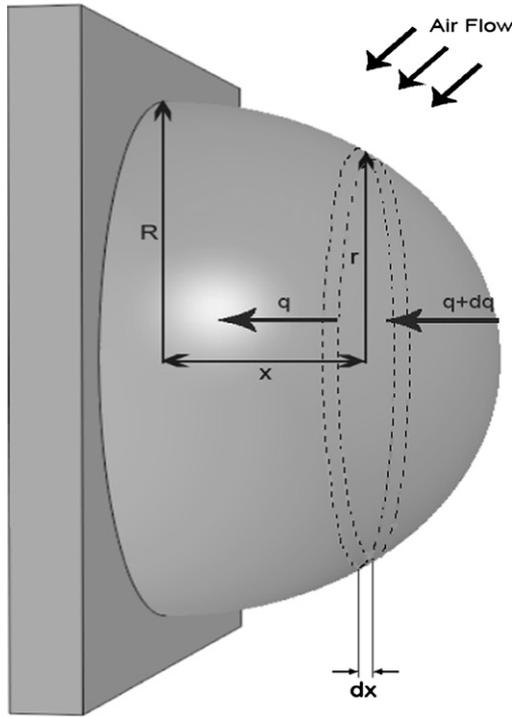
Fig. 1 – Schematic of a fully wet semi-spherical fin.
