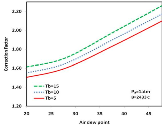
**Fig. 2 – Fin parameter correction factor  $((1 + b_2B)^{1/2})$  as a function of fin base and dew-point temperatures ( $T_{dp}$ ).**
